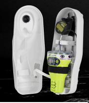
Automatically deploys and activates when a vessel sinks. The beacon floats free once the hydrostatic release is submerged at a depth of 1.5-4.0m (5-13ft). The EPIRB can be manually activated while in it's bracket or when
